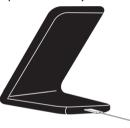
Place your phone horizontal or vertical on the wireless charger. When the phone is being charged, the Smart LED indicator will light up blue automatically to show charging status.
